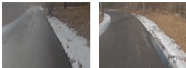
Figure 3: Outtakes from the VISTA driving simulator. When roads do not change in curvature (left), agents may succeed during sensor failures by repeating their last action. When failures occur at changes in road curvature (right), agents must predict curvature based on previous views of the road.
